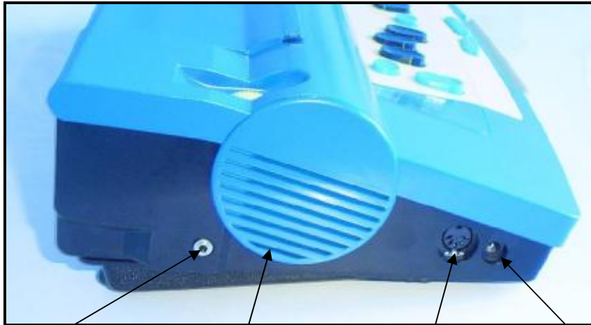
Headphone Jack Speaker Grill AC Mains Power Supply Connector DC Power Adaptor
