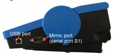
The Mimic port is the second port from the front, on the right-hand side of the MB Pro, and it is the larger of the two ports. You can feel the pins. You can connect either end of the cable to the MB Pro; it is reversible. The connector will only go in one way.
