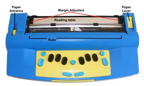
Illustration 5: The top of the MB Pro, cover off, with the Embossing Area labelled right place for your Braille.
