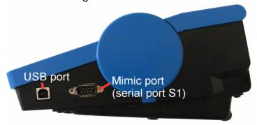
The Mimic port is the second port from the front, on the right-hand side of the MB Writer, and it is the larger of the two ports. You can feel the pins. You can connect either end of the cable to the MB Writer; it is reversible. The connector will only go in one way.
