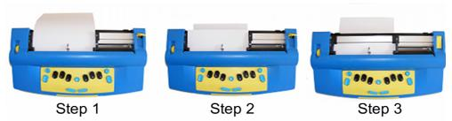
Illustration 8: The three steps for loading paper into the MB Writer
